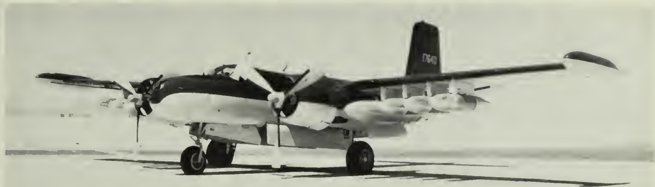
LIGHT bombardment plane, Air Force B-26K, can carry four tons of ordnance under wings besides bomb bay payload.
